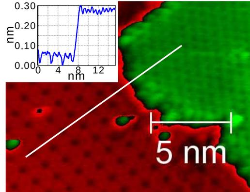
Fig. 1: Detail of the step between first and second silicene layers on  $\text{Ag}(111)$ , in red the first layer, where it is visible the  $\text{Si}_{(h)}3\times 3$ . The second layer in green contains the  $\text{Si}_{(h)}\sqrt{3}\times\sqrt{3}R30^\circ$ .
